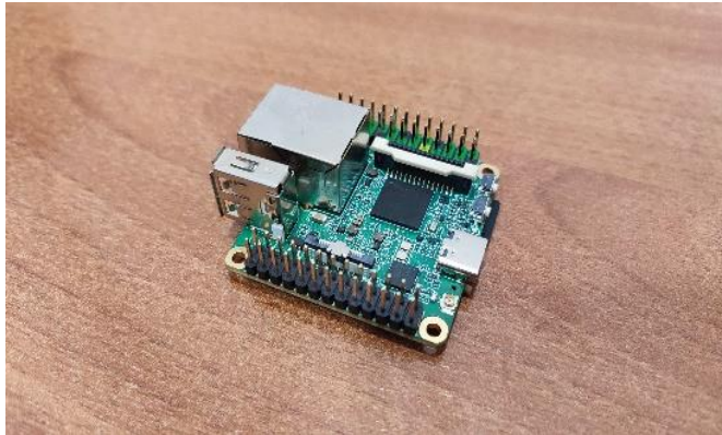
Milk-V Duo S dev. kit (Arm + RISC-V cores) [ https://milkv.io/duo-s ]
